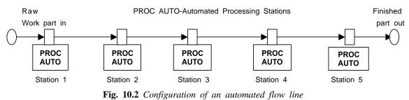
Automated flow lines are generally the most appropriate means of productions in cases of relatively stable product life; high product demand, which requires high rates of production; and where the alternative method of manufacture would invoice large labour content.
